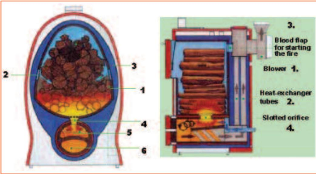
Figure 1: Example of a modern firewood gasifier – the Herlt system.
