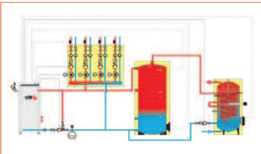
Figure 2: Schematic of a Fröling domestic gasifying system.<sup>1</sup>
