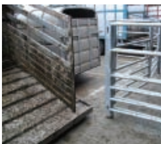
Position the trailer to avoid gaps like this
