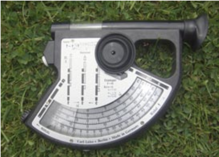
Figure 13. An hypsometer, used for measuring tree height
