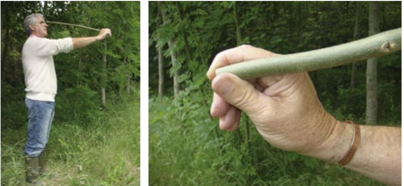
Figure 14. Measuring a stick for use in estimation of tree height
